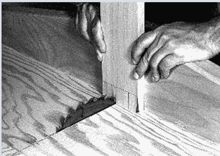
Photo 1- Cut the slots on the ends of the fence base using a table saw cut off box as shown.
