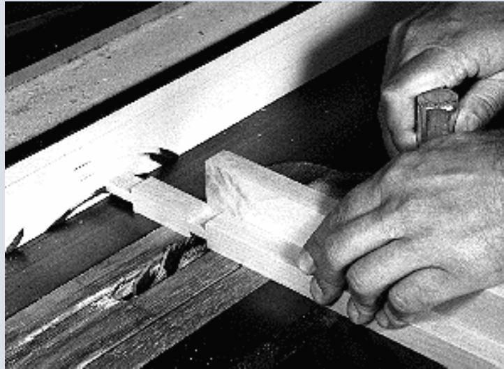
Photo 2- Cut tenons for the lock pieces that hold the side clamps within the slots on the fence base. For safety, make the pieces from long stock as shown. Screw a support fence to your miter gauge to hold the parts as they are cut.
